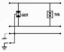
GDT: 3-electrode gas tube TVS: Low-capacitance TVs diode
